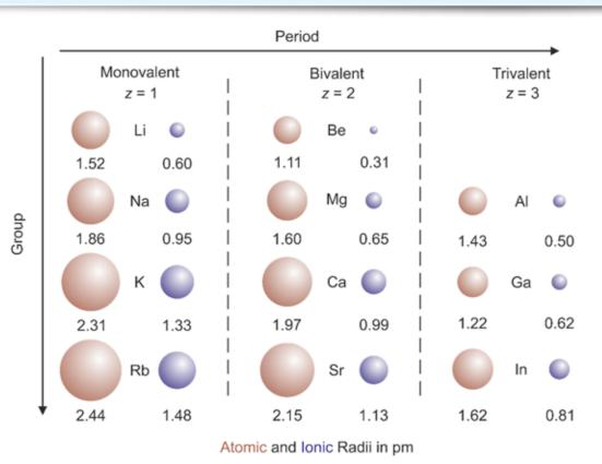
Metals that can be oxidized to multivalent cations offer higher capacity (in Ah) than monovalent cations (Li<sup>+</sup>, Na<sup>+</sup>).
